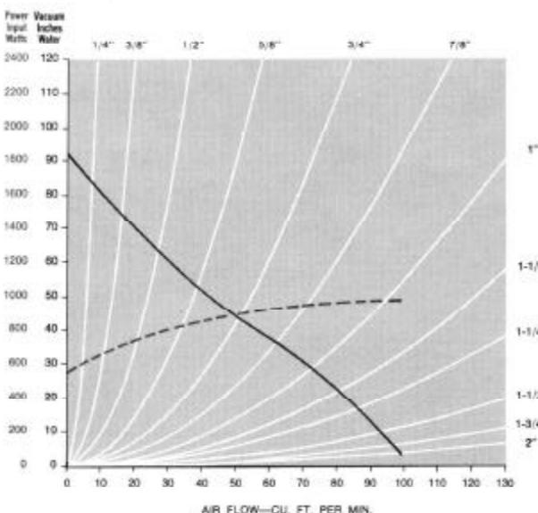
Note: Curves marked with fractional inch designations indicate air flow and vacuum through sharp-edged thin plate test orifices of diameter indicated.
